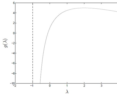
We can verify that the dual function is concave, that its value is equal to  $p^* = 5$  for  $\lambda = 2$ , and less than  $p^*$  for other values of  $\lambda$ .
